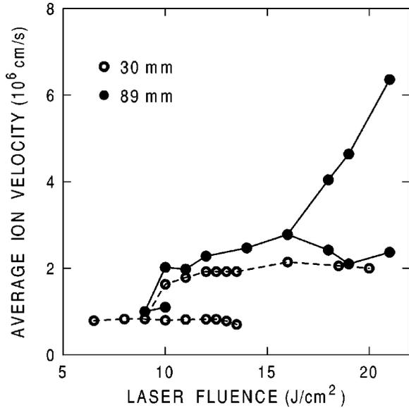
FIG. 4. Average velocity for each peak of ion TOF distributions, measured in vacuum at 30 mm (open points) and 89 mm (closed points) from the target, as a function of laser fluence at 1064 nm. For the double-peaked TOF signals there are two average velocities.
