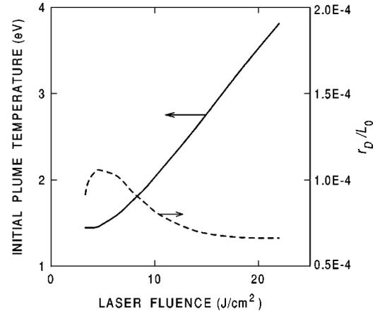
FIG. 7. Calculated values of initial plume temperature (solid line) and ratio of the Debye length to the plume axial dimension  $r_D/L_0$ , realized at the end of 13-ns laser pulse (dashed line), vs fluence for 1064-nm laser ablation of graphite in vacuum.
