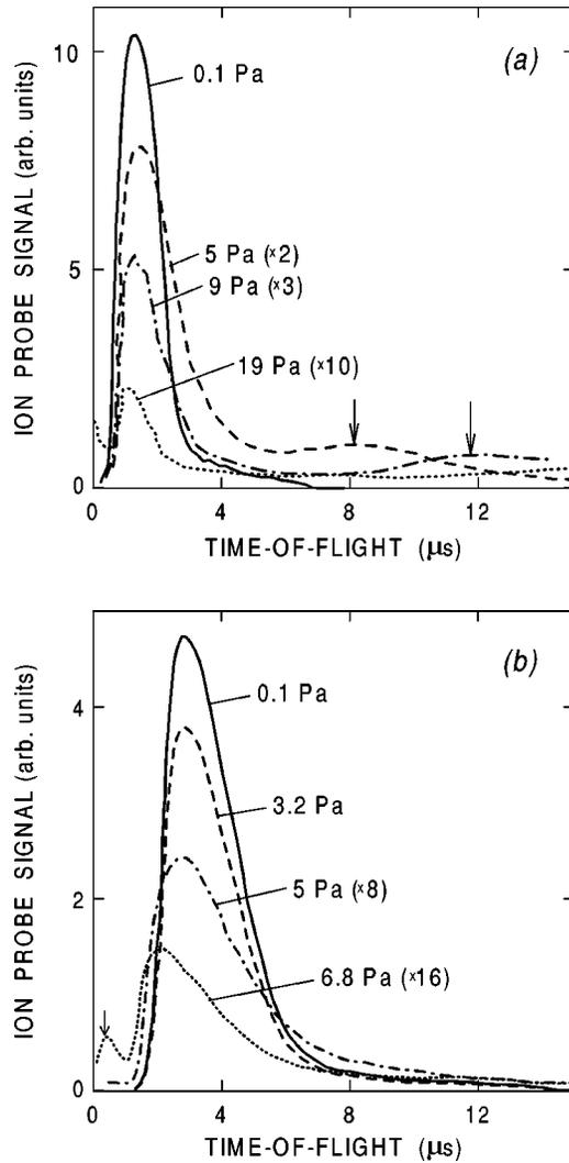
FIG. 13. Ion TOF distributions measured at 30 mm (a) and 89 mm (b) from the target at various background air pressures. Laser fluence is  $25 \text{ J/cm}^2$  at  $1064 \text{ nm}$ . The arrows in (a) show the peaks of slow ions at background pressures of 5 and 9 Pa (at 19 Pa the flux of slow ions peaks at 19.5 ms). The arrow in (b) shows the peak arising due to ionization of the background gas.
