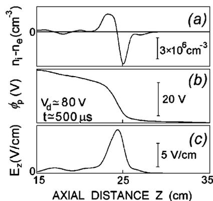
FIG. 1. Example of space charge separation (a), electric potential (b) and electric field (c) profiles across the double layer, adopted from Hairapetian and Stenzel [2].
