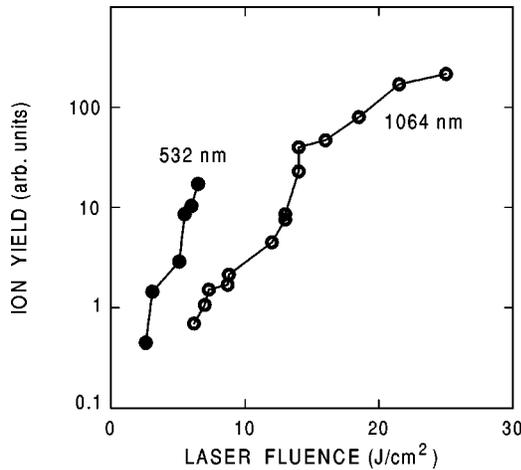
FIG. 11. Ion yield obtained by integrating the TOF distributions collected in vacuum at 30 mm from the target as a function of laser fluence at 1064 nm (open points) and 532 nm (closed points).
