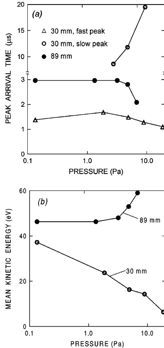
FIG. 14. The most probable arrival time of fast and slow ions (a) and mean kinetic energy of the ions  $\langle E_{kin} \rangle$ , vs background gas pressure. The data are derived from the TOF spectra shown in Figs. 13(a) and 13(b). The  $\langle E_{kin} \rangle$  values are calculated using Eq. (1).
