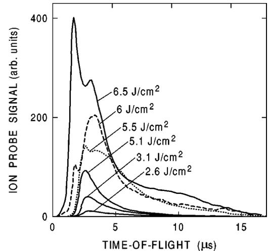
FIG. 12. Ion TOF distributions in vacuum for different laser fluences at 532-nm wavelength. The target-to-collector distance is 30 mm.
