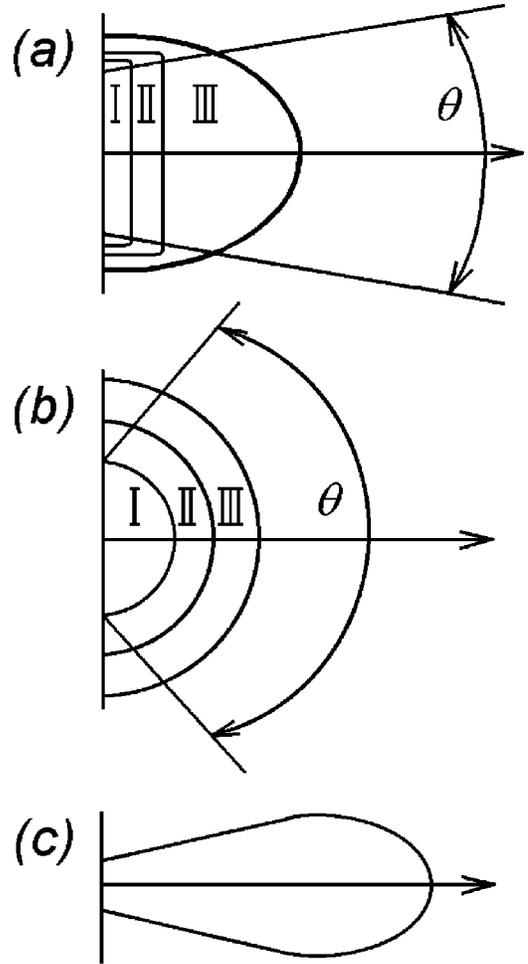
FIG. 9. Schematic representation of DL geometry for three types of initial conditions depending on the relationship between axial and transverse plume dimensions,  $L_0$  and  $R_0$ , at the end of laser pulse: (a)  $L_0 \ll R_0$ , (b)  $L_0 \sim R_0$ , and (c)  $L_0 \gg R_0$ . The designations for the plume regions I–III are used as in Fig. 8. The region II with broken down quasineutrality can be separated by the region IV as in Fig. 8(c).
