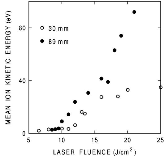
FIG. 5. Mean kinetic energy of ions  $\langle E_{\text{kin}} \rangle$  in vacuum at 30 mm (open points) and 89 mm (closed points) from the target as a function of laser fluence. The  $\langle E_{\text{kin}} \rangle$  values are calculated from the ion TOF distributions (Figs. 2 and 3) using Eq. (1).
